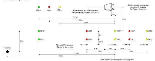
The ramp must be parallel to the jump course and slightly open.
